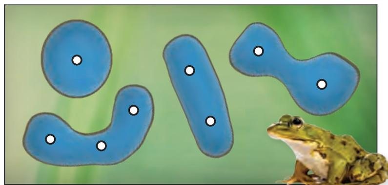
This is a reference to illustrate placement of units to achieve optimal results when aeration is your primary objective. For best results break HP requirements into smaller units and space throughout the water feature.
